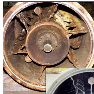
Rotors before and after servicing by LCI.
