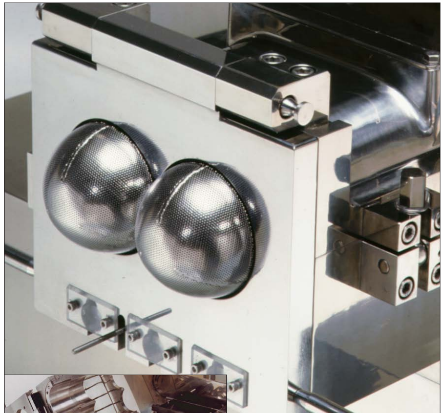
The patented hemispherically shaped dies result in evenly distributed extrusion forces.
