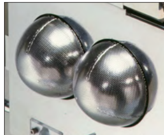
The patented hemispherical shaped dies result in evenly distributed extrusion forces.
