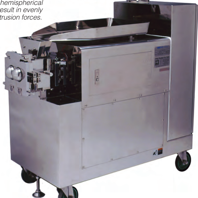
The extrusion chamber with clamshell design opens quickly for easy cleaning and screen changing.
