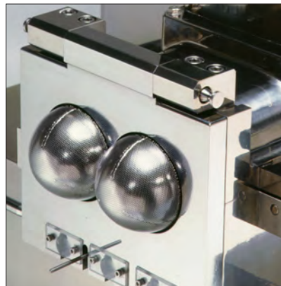
The patented hemispherical shaped dies result in evenly distributed extrusion forces.
