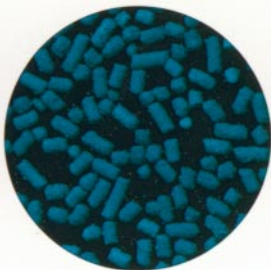
Example showing deformation of extruded pellets to produce spheres
