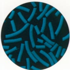
Example showing deformation of extruded pellets to produce spheres
