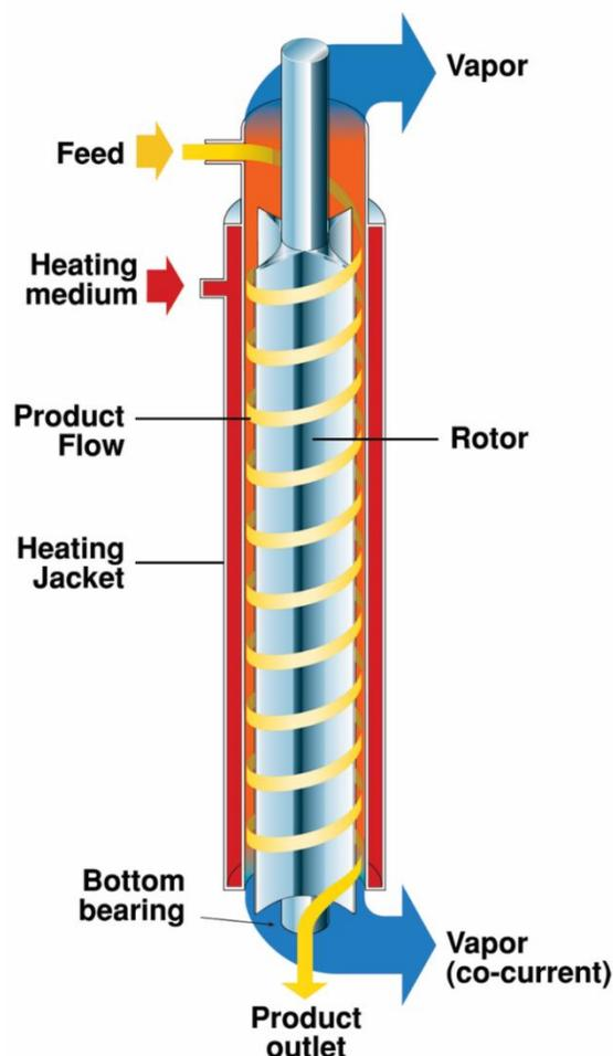
**Figure 2: Agitated Thin-Film Evaporator Internal Cross-section**
