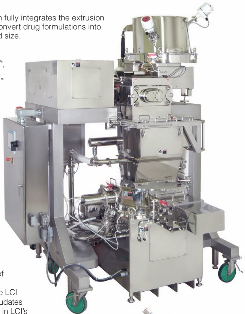
Above: LCI's Continuous Drug Pelleting System shown with the Radial Xtruder Model EXDS-100G, Discharge Device Model CD-30, and Marumerizer Model QJ-700TG.
