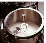
Above: Twin Bowl Marumerizer system. Left: Systems are available with either manual or automatic integrated plate lifting devices.
