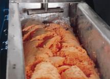
Twin shafts with special blades thoroughly mix powders and liquids
