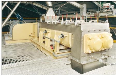
The LCI Kneader provides a homogeneous mix of liquids and powders
