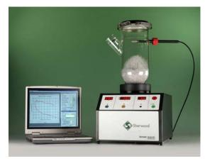
Lab Scale Fluid Bed Dryer
