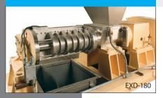
Production scale twin screw extruders available in cabinet style or flat bed models
