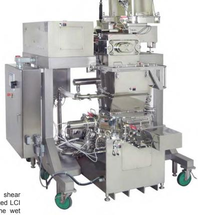
Above: LCI's Continuous Drug Pelleting System shown with the Radial Xtruder Model EXDS-100G, Discharge Device Model CD-30, and Marumerizer Model QJ-700TG.
