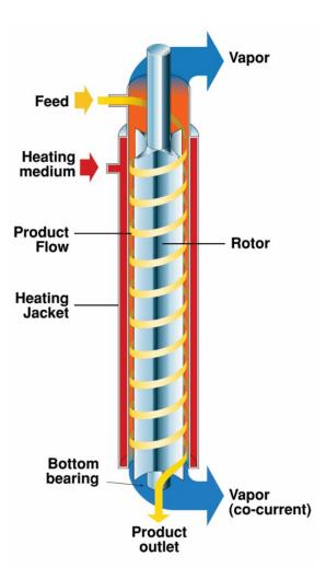
Figure 2: Agitated Thin-Film Evaporator Internal Cross-section
