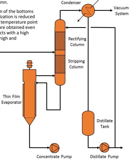
Figure 1: Typical Equipment Combination For the separation of a lighter boiling component, so that the heavy boiling component is obtained in as pure of a state as possible; continuous operation under vacuum
