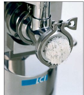
Three types of extrusion—axial, radial, and dome—can be evaluated by simply changing the extrusion head.
