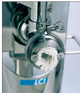
Three types of extrusion—axial, radial, and dome—can be evaluated by simply changing the extrusion head.
