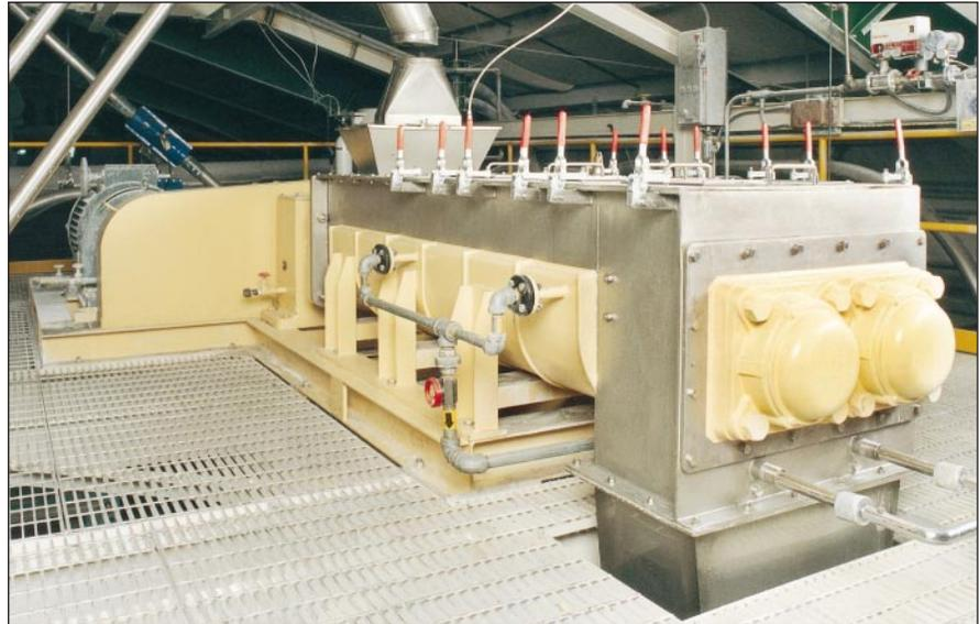
The LCI Kneader provides a homogeneous mix of liquids and powders
