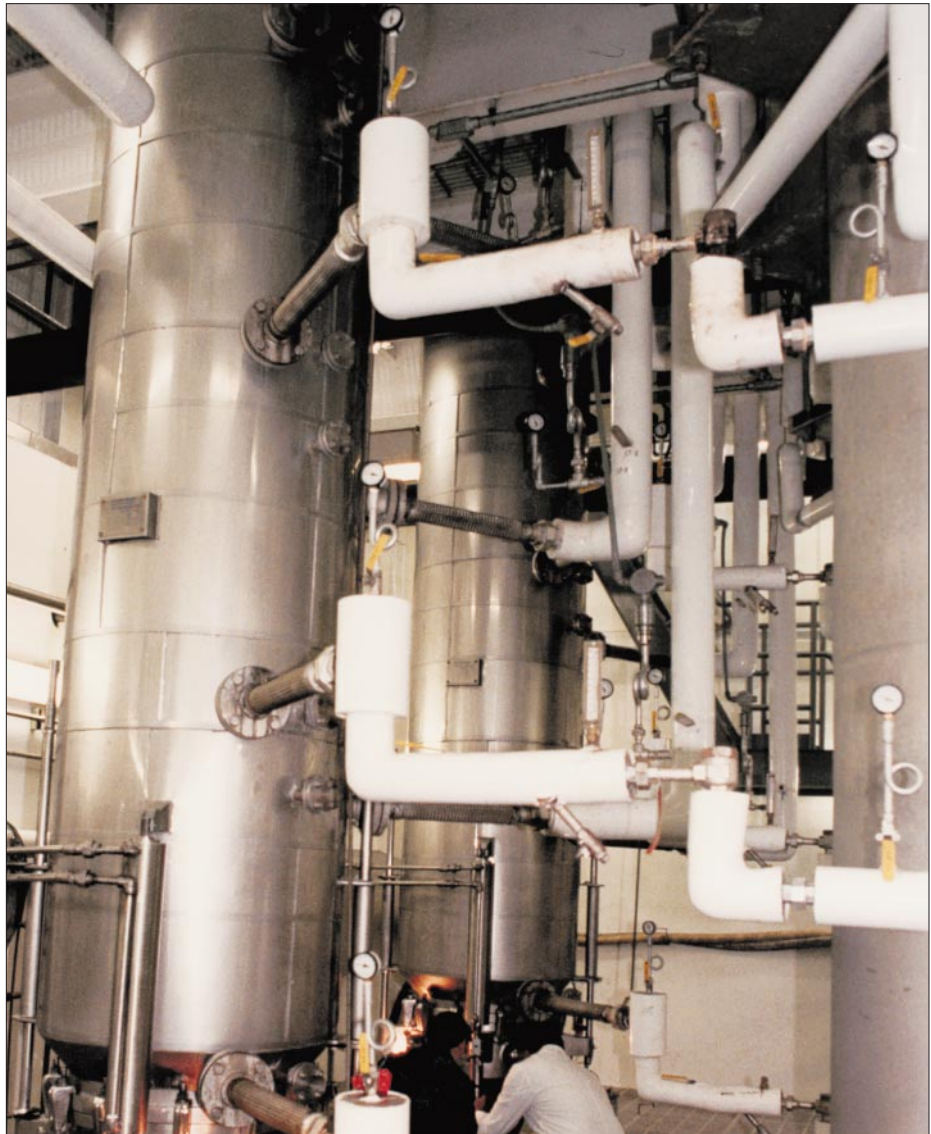
LCI Thin-film Evaporation Systems Concentrating Viscous Food Product
