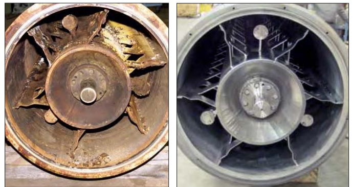
These before and after photos show how used feed screws can be returned to like-new condition.
