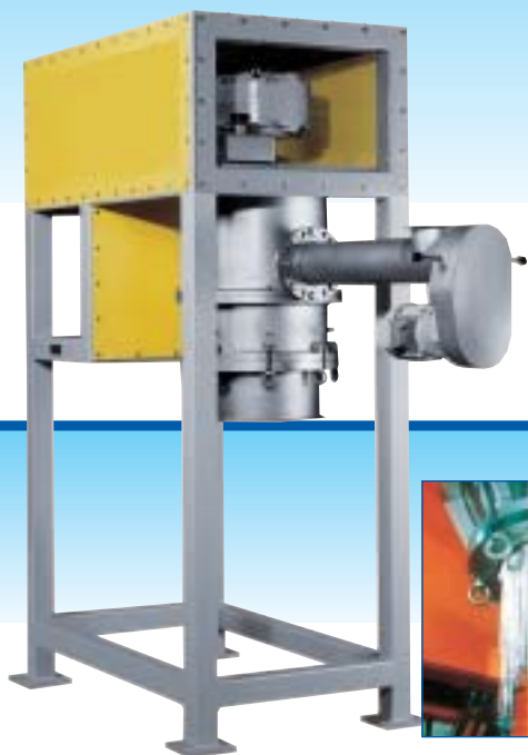
▲ Press 24-390 with overhead drive for pelleting pasty products
