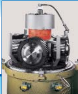
▼ Press with hydraulic nut, positive roller drive, and die heating for plastic additives.
