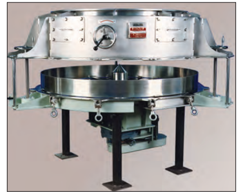
Sanitary designs feature high internal polishing and hinged or lift-type upper case for cleaning access.
