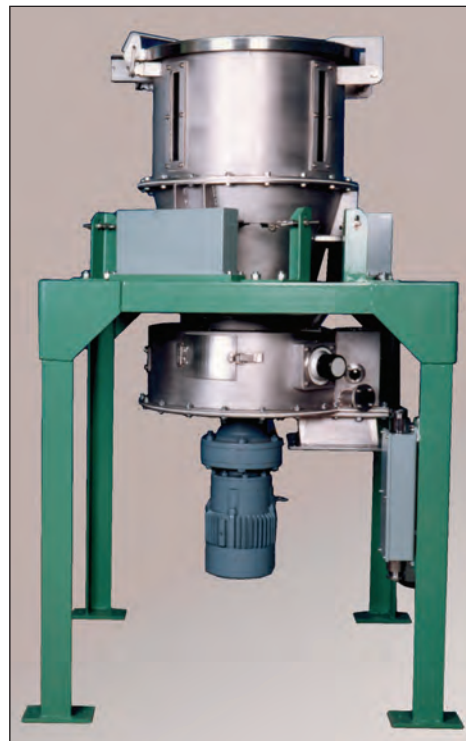
Loss-in-weight control is achieved by monitoring the weight of the material being discharged and automatically adjusting the rotation speed to achieve the desired rate.
