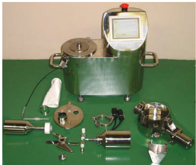
The SPG-2 can be easily disassembled for cleaning and validation
